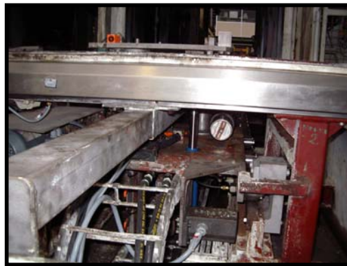
Multi-Point system with a reusable MEMOLUB lubricator.
