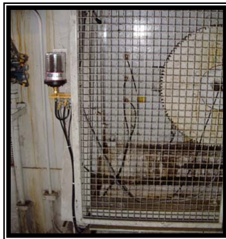
Multi-Point system with a reusable MEMOLUB lubricator.
